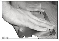
**7.2.3** Fold down the foldable flange of the adapter/damper. This flange must be at  $90^{\circ}$  from the remaining flanges. See picture beside.
